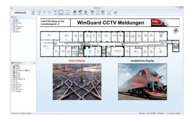
Depending on the addressing of the various operator stations, individual displays can be created and assigned. This ensures a smooth event processing anytime.
