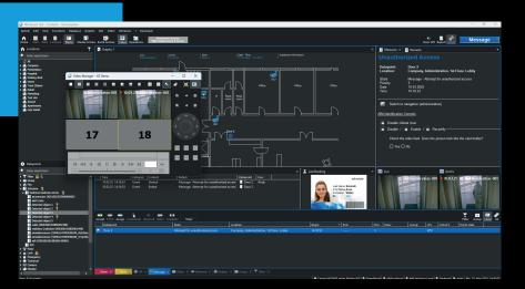
PSIM solutions provide security teams with instant alerts about suspicious activities, such as unauthorised after-hours access or anomalous user journeys. The integrated combination of AIM and WinGuard leverages real-time data to enable automated workflows that guide rapid incident response.
